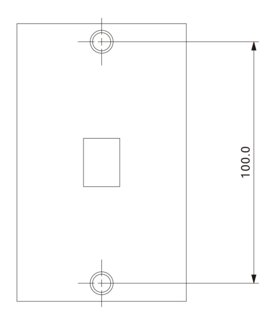
Note: Φ8\*40 expansion tube with M5\*40 tapping screw is recommended
