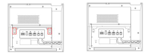
2. Insert the wall mount bracket into the rear housing slot (where the bracket spindle was originally fitted)
