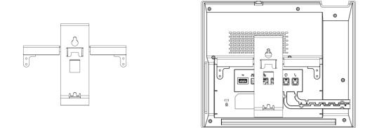
3. Locking screws fixing (use screws removed in step 1)
