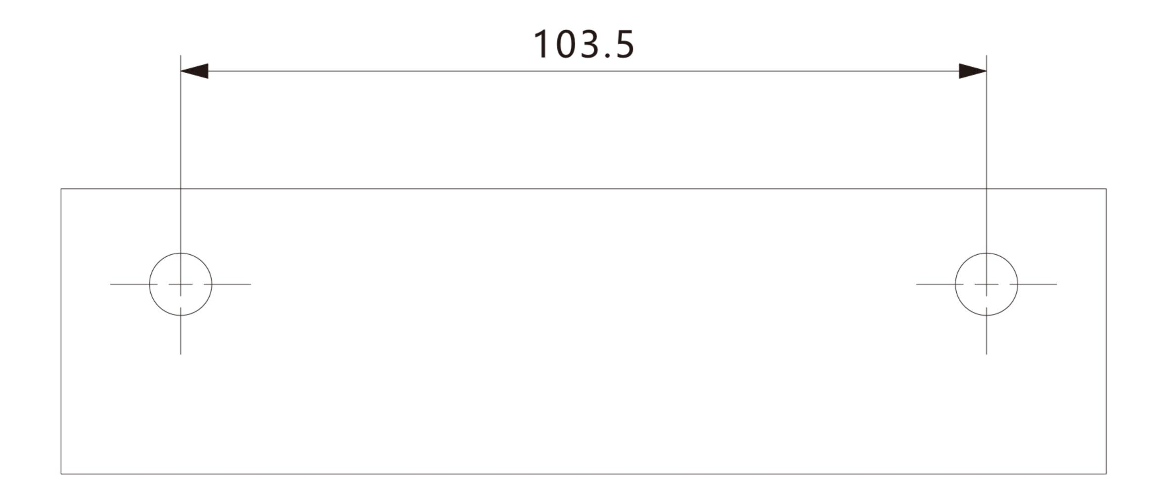
Note: Φ6\*40 expansion tube with M4\*40 tapping screw is recommended
