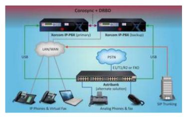
Blue Steel CXTS3000 – TwinStar Plus configuration featuring dual Blue Steel CXT3000 servers with optional Astribank included.
