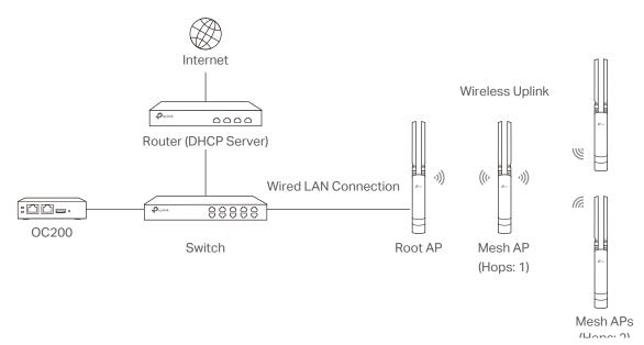
After all the EAPs are adopted, a mesh network is established. Then the EAPs connected to the network wirelessly also can broadcast SSIDs and relay network traffic to and from the network through the uplink AP.
